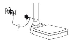
Please use only the mains unit supplied or mains units from the seca range of accessories. Before plugging the unit into the socket, check whether the mains voltage marked on the mains unit matches local mains voltage.
